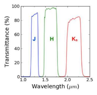
Fig. 3.1 Photometric filters used for the GALACTICNUCLEUS survey.
