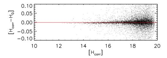
**Fig. 4.2** Difference in H-band photometry before and after applying the distortion solution. The results of the photometry computed before and after the application of the distortion solution are indicated by  $H_0$  and  $H_{corr}$ , respectively. This plot corresponds to detector #3 of F1 data. The units are magnitudes, with the zero point being the one specified in the HAWK-I user manual.
