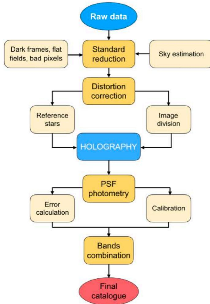
**Fig. 5.7** Scheme of the obtention of the final catalogue for each chip.
