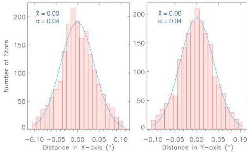
**Fig. 4.1** Goodness of the distortion solution (detector #2 *H*-band F1 data). Differences in arcseconds between the relative positions of stars in the corrected HAWK-I frames and in the VVV reference image. Left panel X-axis and right panel Y-axis. The blue lines are Gaussian fits to the histograms. For both histograms, the centre of the fit lies at 0.0 arcseconds, with  $\sigma = 0.04$  arcseconds.
