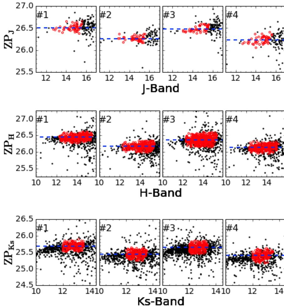
**Fig. 5.4** Zero point calibration for each chip and band in F1 data. Black points represent stars common to the SIRIUS catalogue and our final list. Red points mark the stars used to compute the zero points. The mean zero points are indicated by the blue lines. The systematic deviations for the brightest stars are due to saturation.
