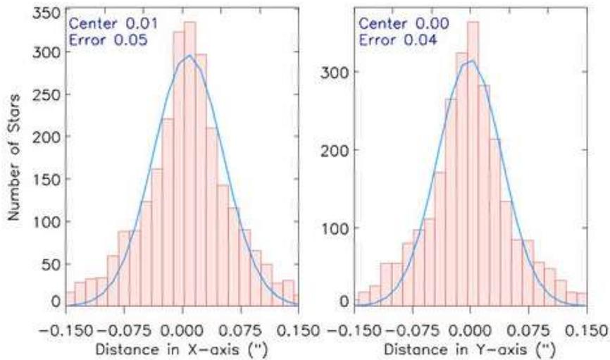
**Fig. 5.3** Position accuracy. Differences in arcseconds between the positions of stars in the final HAWK-I chip #4 (F1  $H$ -band) and in the VVV reference image. Left panel X-axis and right panel Y-axis. The mean and standard deviation are  $0.01 \pm 0.05''$  in X and  $0.00 \pm 0.04''$  in Y.
