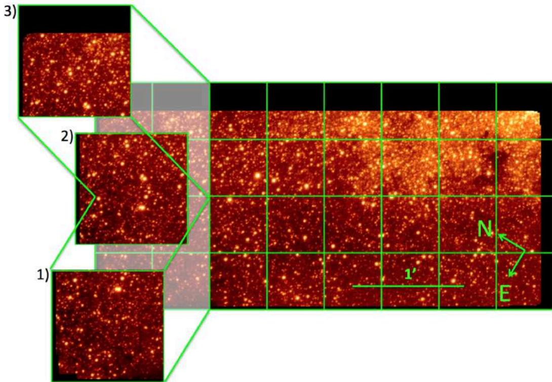
**Fig. 4.3** Long exposure image (*H*-band chip1, F1 data) divided to obtain the sub-regions used in the holographic procedure. Region 2) corresponds to an overlapping region between 1) and 3) showing the overlapping strategy described in the text. The green lines show the division of the rest of the detector.
